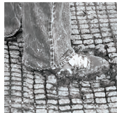
Image 1: The Snowshoe Effect – Tensor TriAx and BX Geogrids distribute heavy loads over soft soils just like a snowshoe supports the weight of a man over soft snow.
