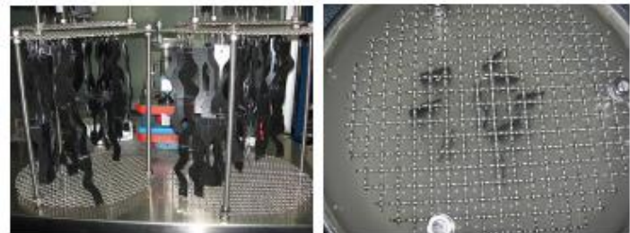
Figure 2. Pre-cut specimens in special sample holders and immersed in the brine solution.
